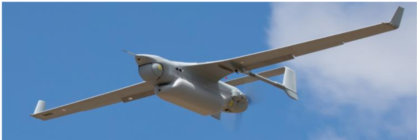
Insitu Integrator RPAS – 4.8 metre wingspan, cruise speed 60 – 80 kts
