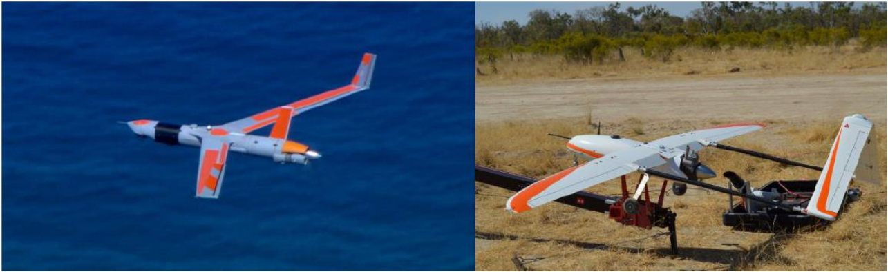
Insitu ScanEagle RPAS (left) and Insitu Pacific CT220 RPAS (right) – 3.1 metre wingspan, cruise speed 45 – 60 kts
